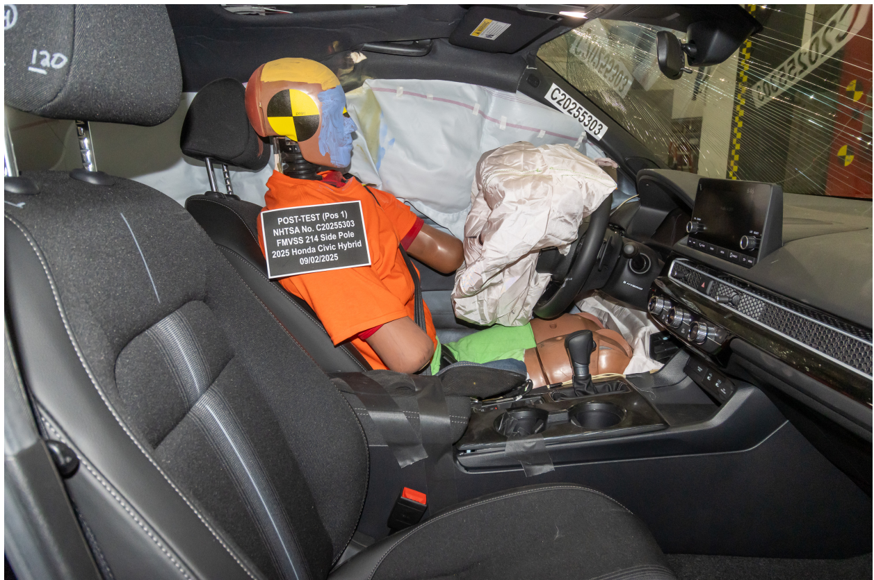
Figure A-12: Post-Test Dummy Through Opposite Window
